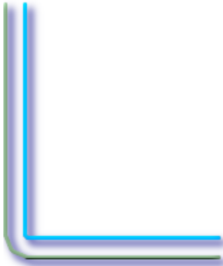
15, 'quad_segs=4 join=bevel' shown with original line
