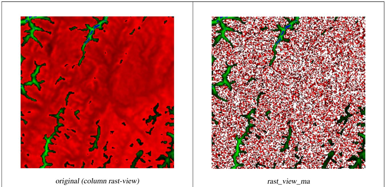
Create a new 3 band raster same pixel type from our original 3 band raster with first band altered by map algebra and remaining 2 bands unaltered.
