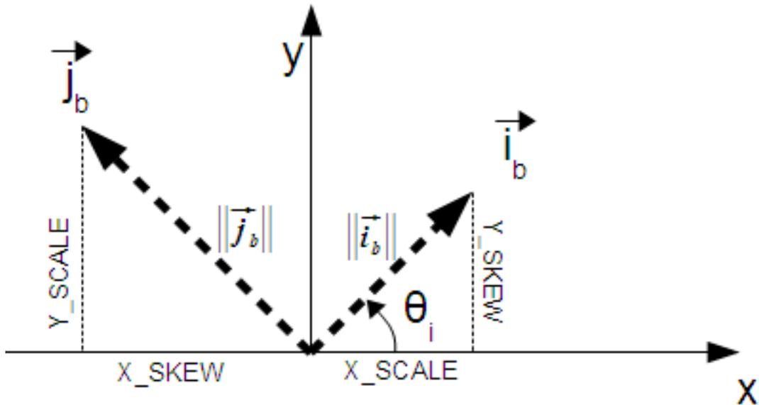
*Pixel Width: Pixel size in the i direction*
