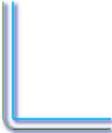
15, 'quad_segs=4 join=bevel' shown with original line
