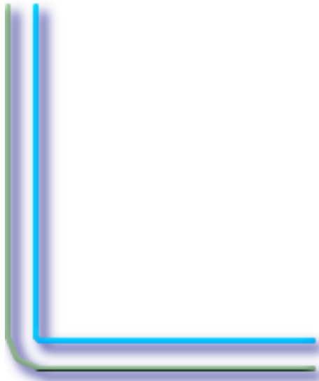
15, 'quad_segs=4 join=bevel' shown with original line
